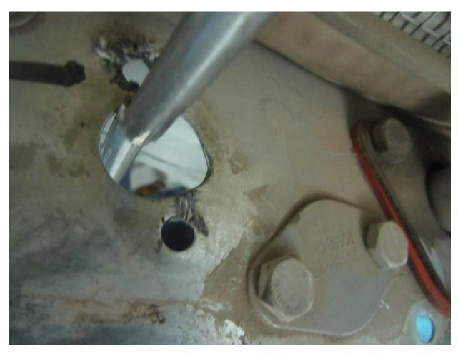
Teledyne Continental, IO-240-B Corroded Weld on Oil Sump Causing Leak
